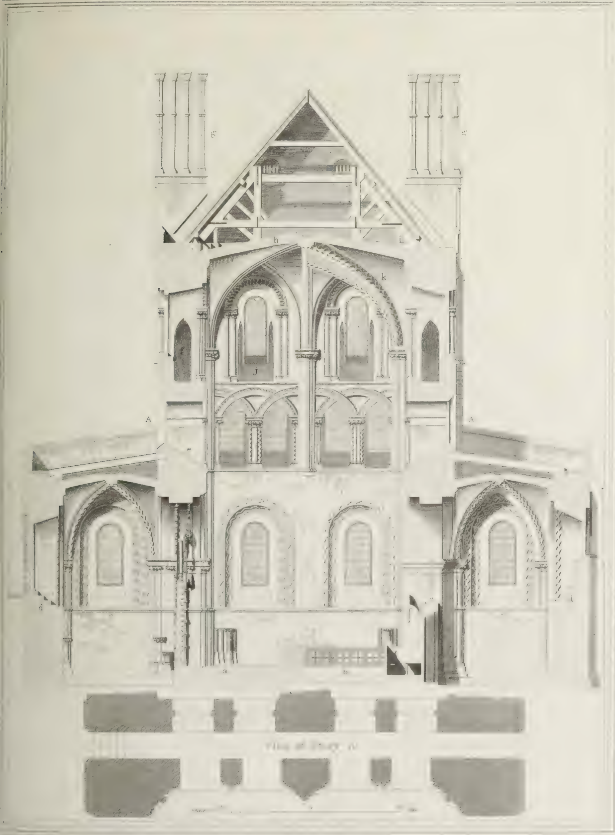
SECTION OF ST. BARTHOLOMEW'S CHURCH, LONDON (FROM A DRAWING BY J. NICHOLS)
